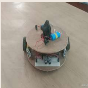
Model Making - a dust cleaning robot using Arduino Uno Department of Electronics
