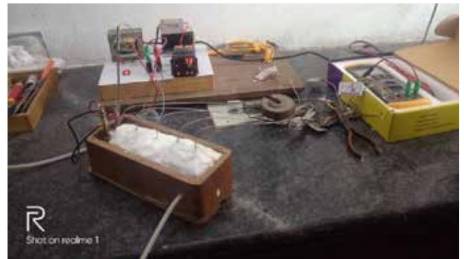
Figure 1: the experimental set up for Thermal Conductivity by Searle's method
